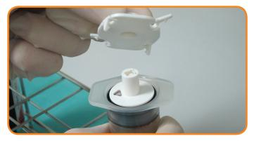
**4.** Take off guide plate by rotating it 90°. Place triangular port on the side of the syringe where serum is the deepest by rotating the base of the syringe plunger. Work carefully to not disturb the clot.
