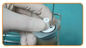
Connect cannula to a 35mL syringe. Penetrate the black stopper through accessory port and carefully aspirate ACS, being careful to not aspirate any RBCs.
